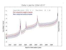
The  $\Delta V$  necessary to avoid the 2102 collision of 2004 VD<sub>17</sub> with the Earth (Carusi 2005); even the very distant 2032, 2041 and 2067 encounters lower  $\Delta V$  significantly.
